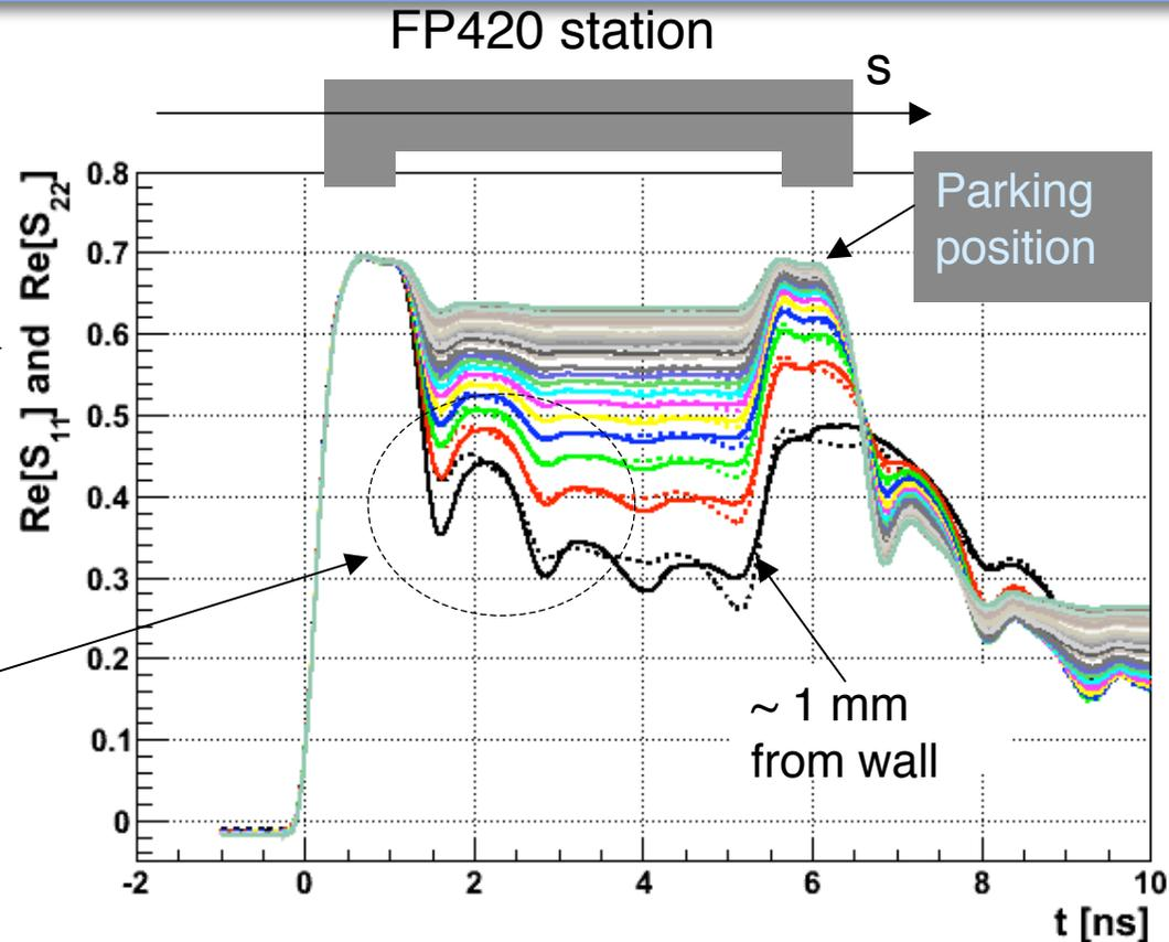
This signals can be used to estimate **line impedance** to be used in the “log formula”
