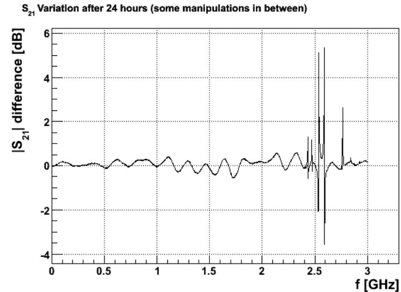
$S_{21}$  measured in two different days with “manipulations” in between
