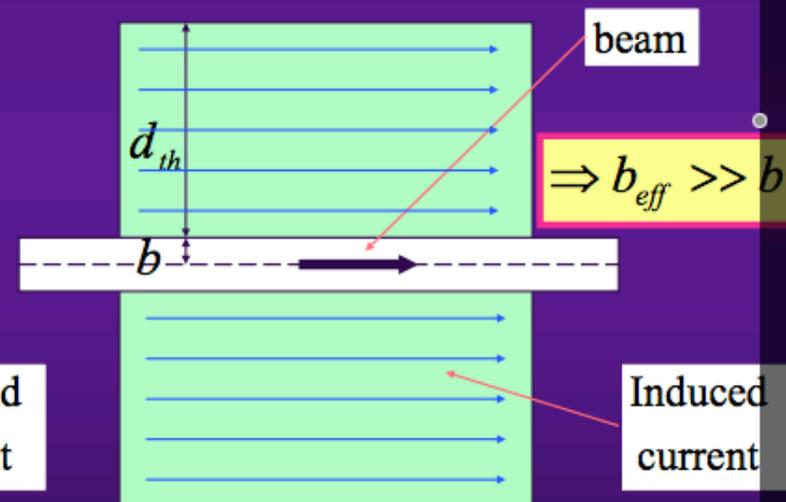
$\Rightarrow$  **This inductive by-pass effect is therefore observed even with a single layer extending up to infinity**
