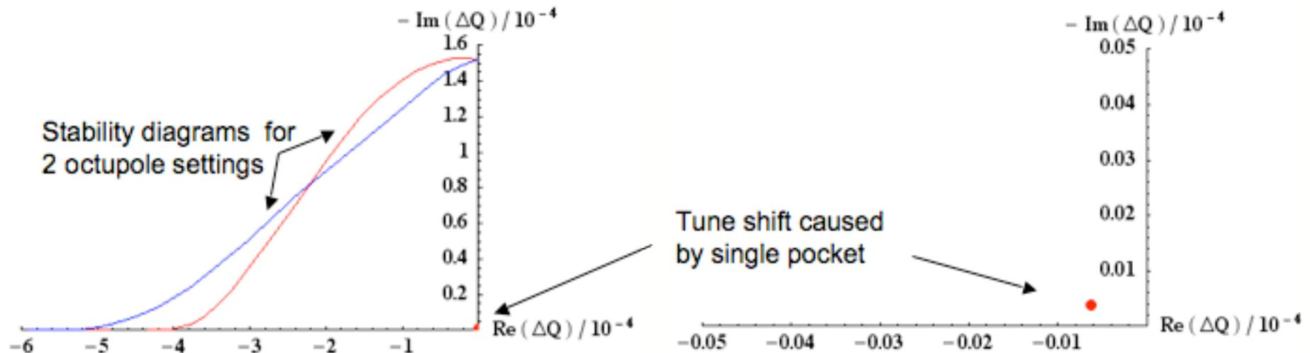
Plots produced using E.Metral's model applied to one FP420 station
