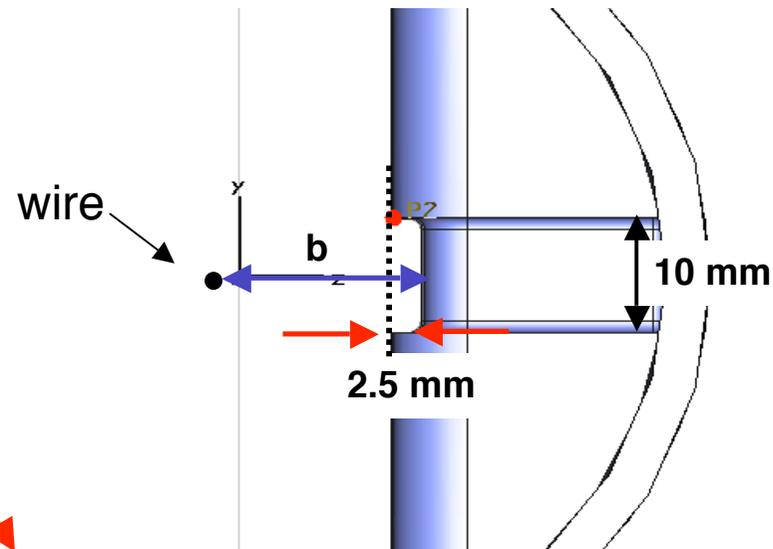
$\sim 0.5$  mm = correction to apply to mechanical position measurement
