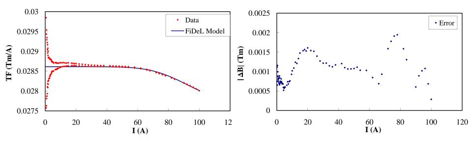
Example of the MCBC : note that the hysteresis was not modeled in this case. It is then necessary to evaluate the relevance of this effect.
