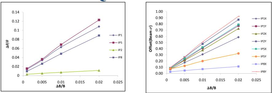
To have an idea on how precise the model should be we can look at how the orbit evolves with the field errors. Those plots show the effect of the field error on the crossing angle (left) and position (right) => a model with a precision of ~0.2% should be enough to get errors of the same order as the ones from the beam-beam effect.
