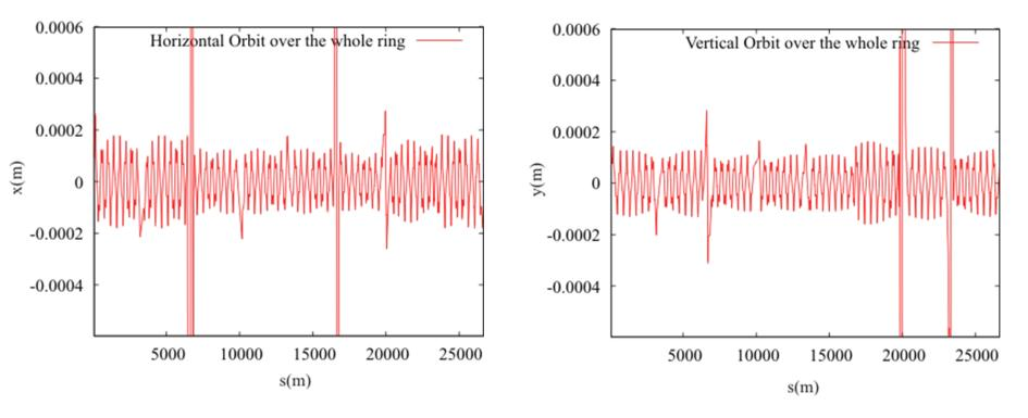
By adding the MCBX errors we generate a residual orbit with  $\sim 0.07$  mm in x and  $\sim 0.06$  mm in y in this case( rms outside crossing angles).
