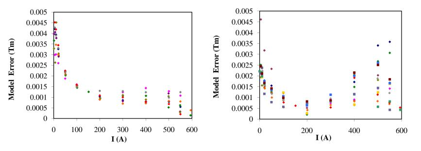
If we now look at the errors in the MCBX we can see that the order of magnitude is ~5 times larger than the one in the MCBC/Y.  $\Rightarrow$  The orbit errors are also larger : approximately 1 $\sigma$  in position and 10% in angle in the worst case (15 $\mu$ rad at IP5).
