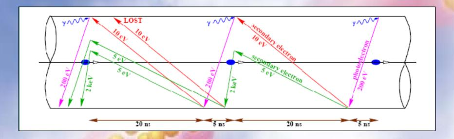
Photoemission, residual gas ionization and secondary emission give rise to a quasi-stationary electron cloud inside the beam pipe !!!
