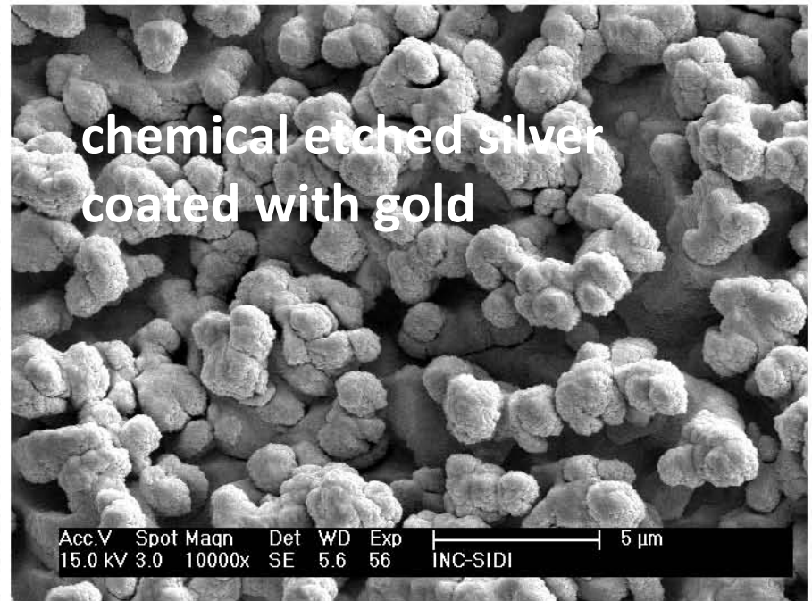
Fig. 13. SEM images of the effect of gold coating a chemical-etched silver sample. Effect of coating with 2 μm Au. Left, MP etched Ag sample; right, same after Au coating. The type of roughness has significantly changed. Samples MP were representative (witness) of multipactor sample waveguide halves, see Fig. 14 . The substrates were of 20μm-Ag-plated aluminium from Tesat.
