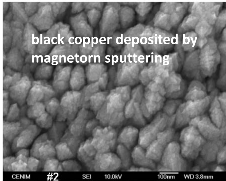
Fig. 3. SEM images of rough “black” copper deposited by magnetron sputtering. Samples #2 and #7, deposited at relatively high pressure and rate for separate columnar growth. Sample #7, deposited over single crystal Si wafer, was cleaved and its profile examined.
