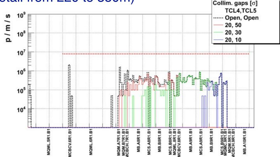
Indeed TCL5 at 10-20 sigma reduces the losses, but even at 30 and 50 sigma losses at B8 (concern for Baichev-Jeanneret) are reduced(remember log scale)
