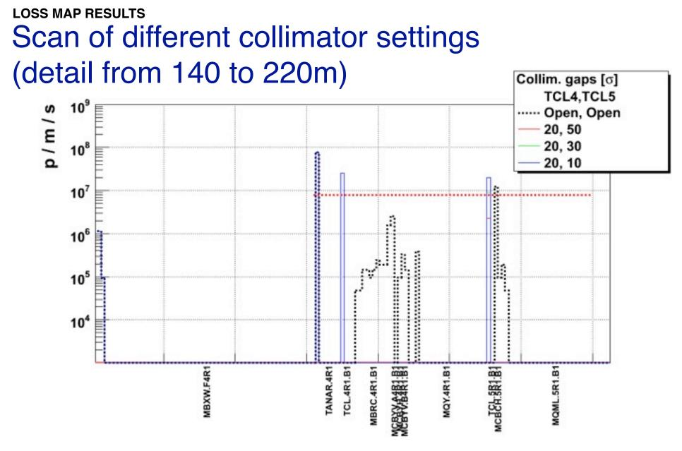
Important: TCL4 at 20 sigma and TCL5 at 50 sigma are enough to protect Q5 (all the job is done by Q4 actually)
