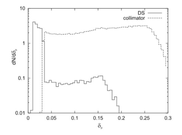
Figure 3: The momentum distributions of the lost protons. Dashed histogram - the protons intercepted by the collimator, solid one - those one lost in the dispersion suppressor and in the arc cells, including the protons which are reemitted by the collimator.
