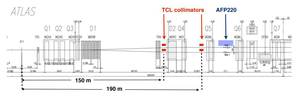
TCL4 and TCL5 are designed to protect D2, Q4, Q5, Q6 (and possibly other downstream elements down to the beginning of the arc) and RR regions from physics debris particles during high luminosity runs (L > 2e33)
