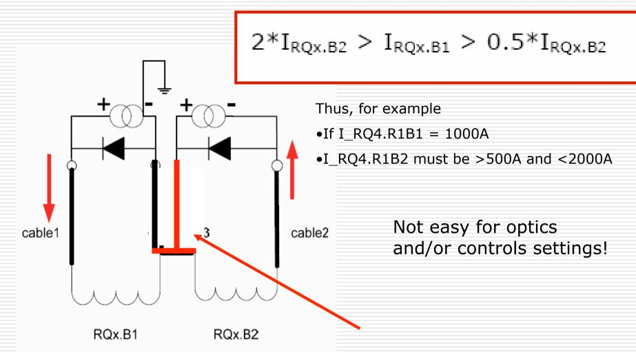
Constraint is removed if an extra cable is added
