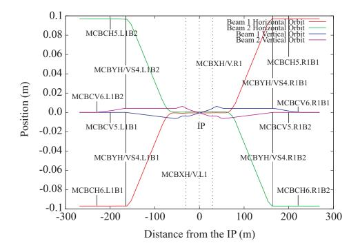
MCBX in triplet - important for crossing angle and aperture at injection
