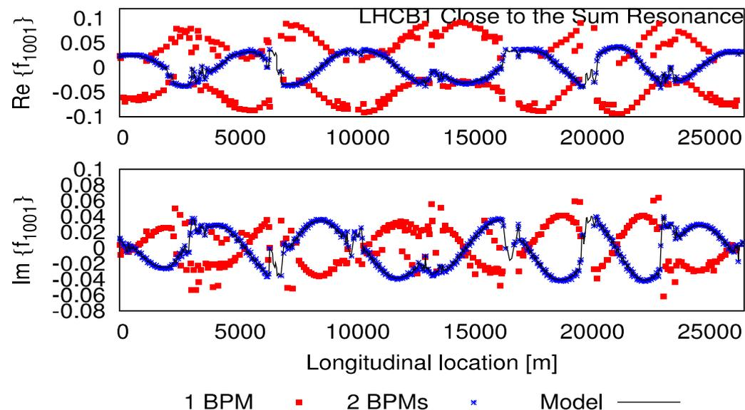
In order to be able to measure in this configuration we asked to equip BPMs close to Q7, which gives good phase advance to the BPM at Q1 (at least at injection)
