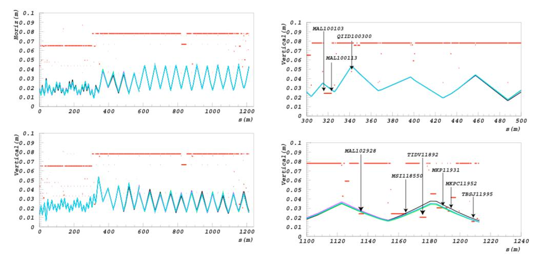
All five slices with epsx=0.5 um, epsy=0.75 um dp/p=0.5e-3 Beam enveloppes are practically superimposed on this scale
