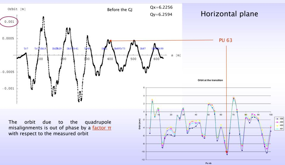
The quadrupole misalignments are not a sufficient explanation to find the same order of magnitude (x[Pu63] = -10 mm at the transition instead of 0.5 mm calculated by simulation)
