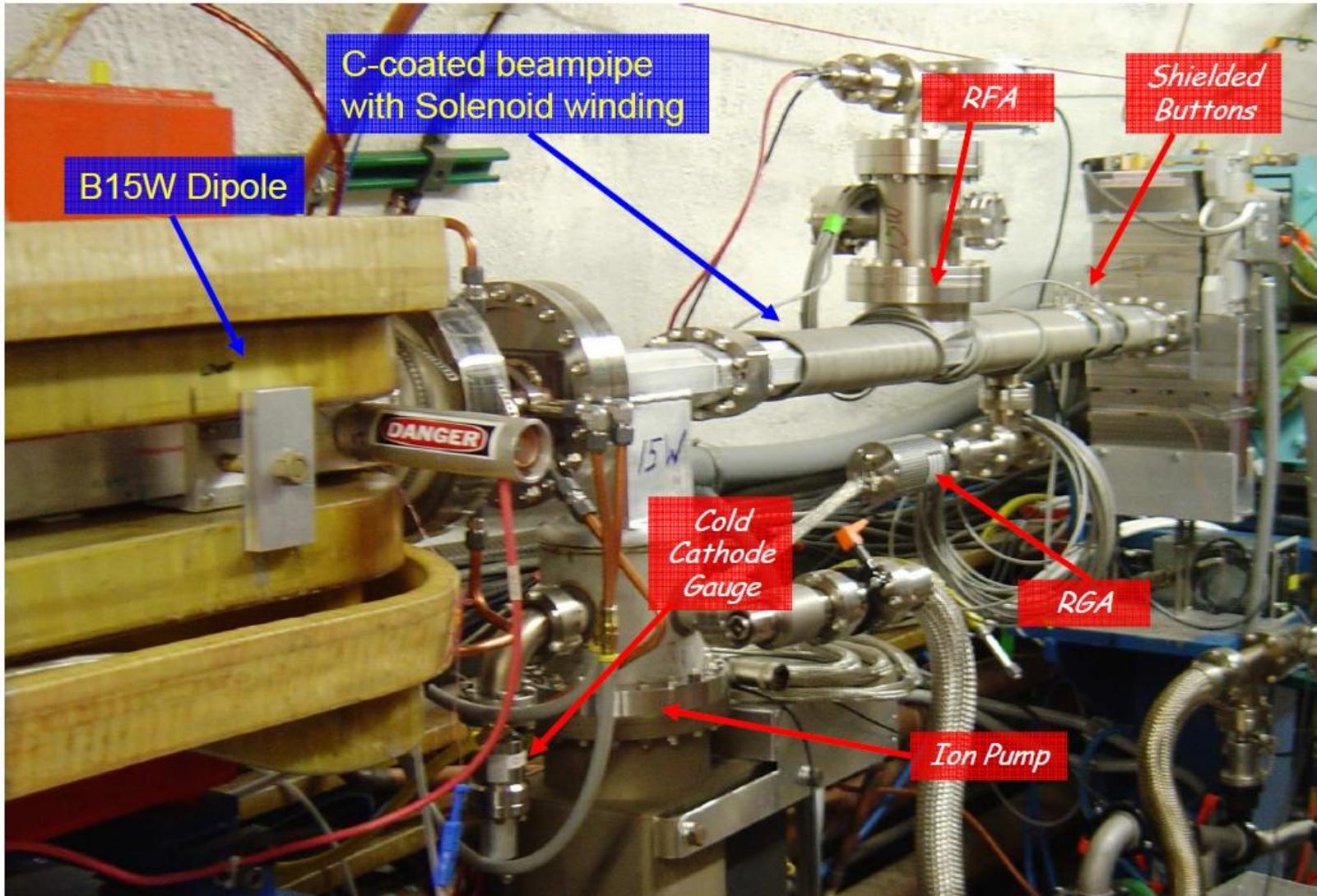
Initial SEY of a-C coating = 0.98 (measured on witness samples)
