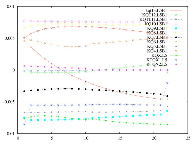
Normalised strength, left side ir ip5. 21 steps, each 10 % reduction in β. Last step is target strength.
