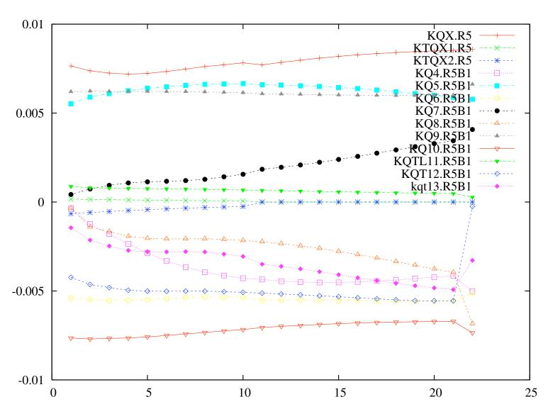
Normalised strength, right side. 21 steps, each 10 % reduction in β. Last step is target strength.
