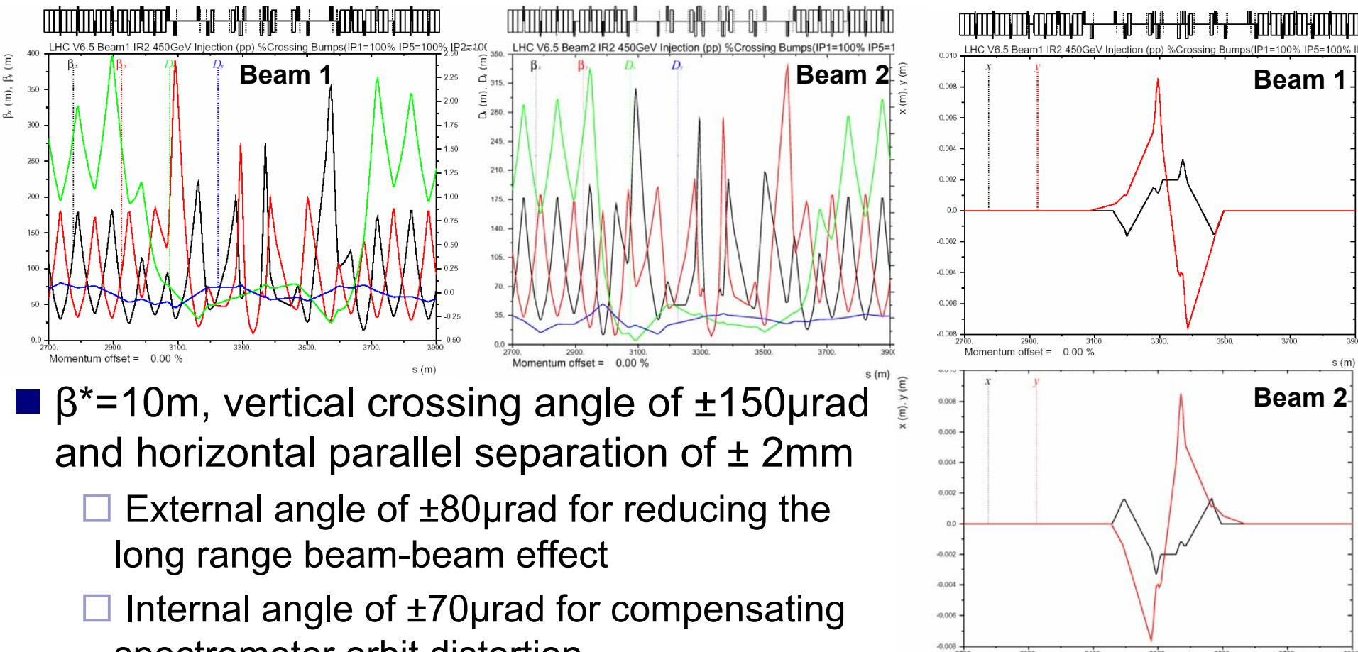
■  $\beta^*=10\text{m}$ , vertical crossing angle of  $\pm 150\mu\text{rad}$  and horizontal parallel separation of  $\pm 2\text{mm}$
