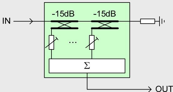
“Sampled line” type comb filter (8 sections):
