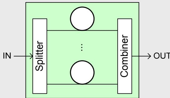
“Delay line” type comb filter:
