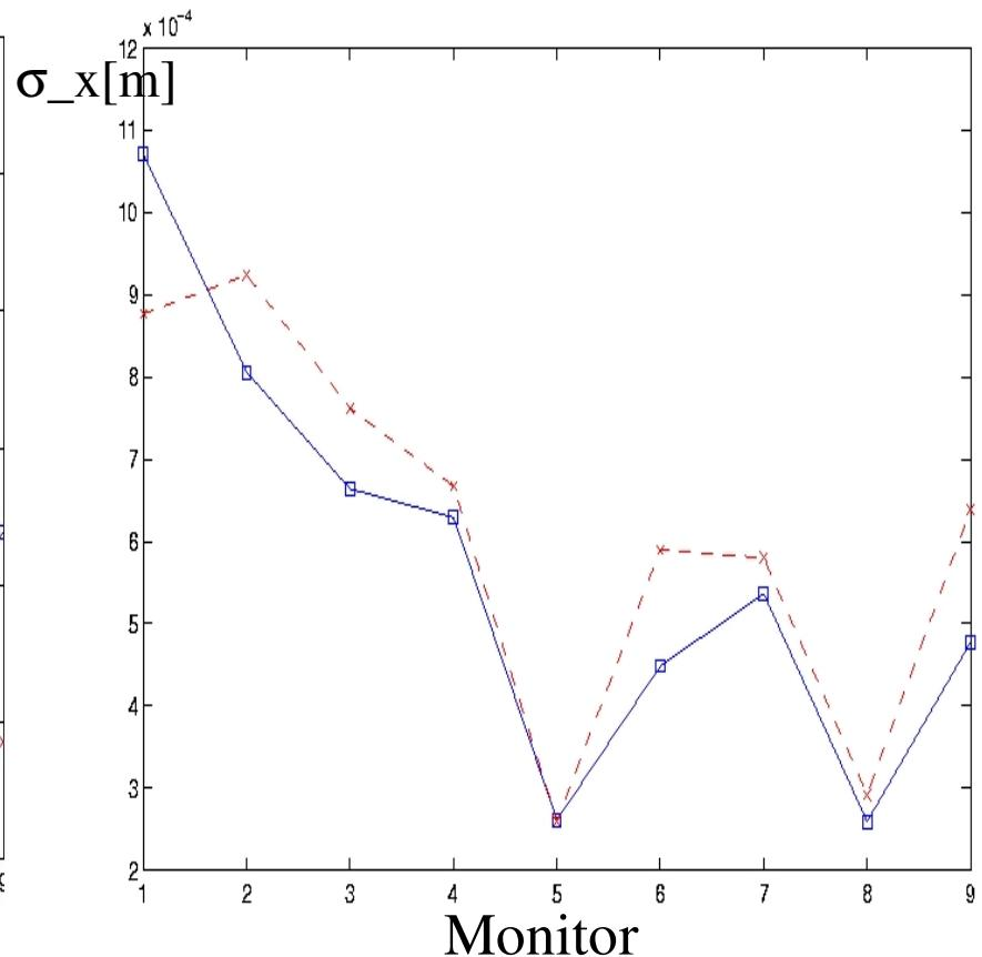
Comparison to mad (in blue) – an individual measurement (left) and average over 1h (right, distribution cut at 5 sigma)
