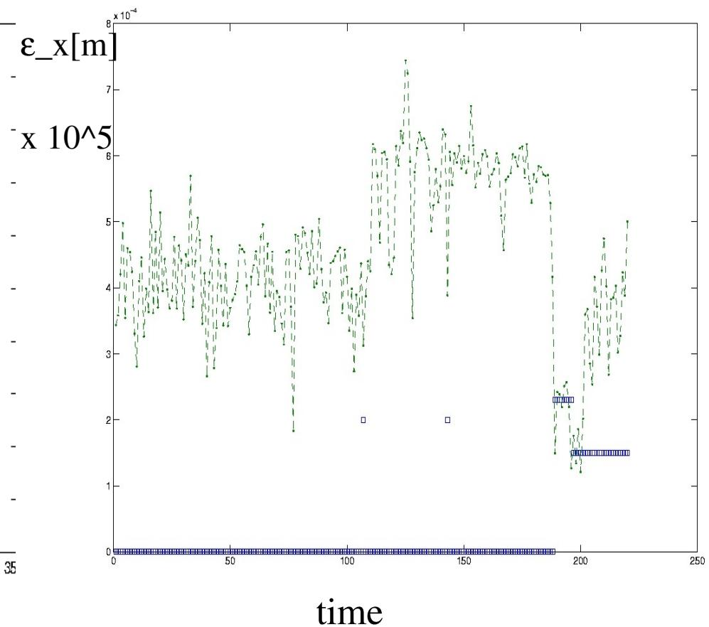
Emittance x all (left) and a relatively good piece of data (right, scaled  $10^5$ ). Dp/p recorded by the emittance matching program on the right plot in blue
