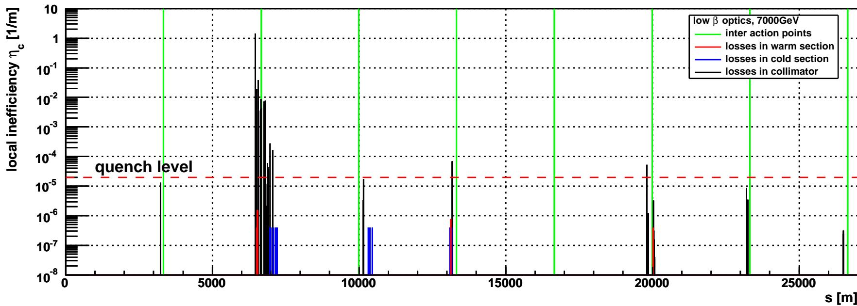
Copper secondaries set to nominal settings, carbon secondaries set to relaxed opening ( $26.5\sigma$ ), cryogenic collimators (material copper, length 1 m) placed at 300 m and 387 m from IR7 at  $15\sigma$ .
