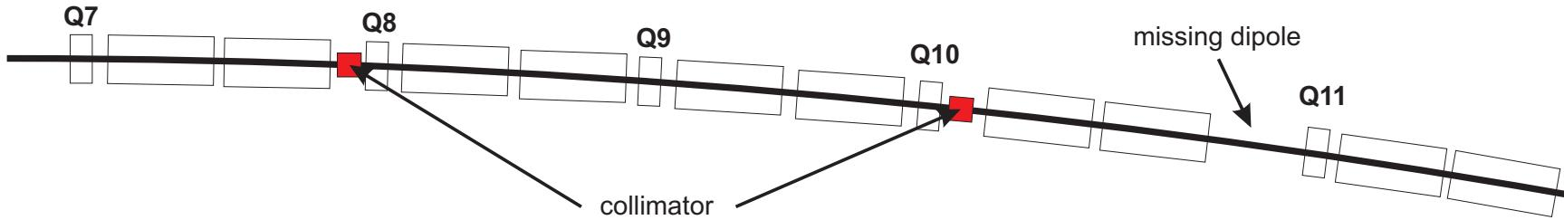
symmetric shift of two dipoles at the beginning and end of the dispersion suppressor by 3 m.
