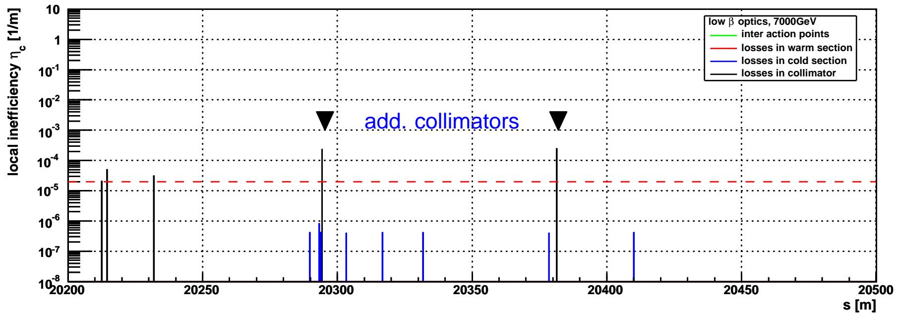
Copper secondaries set to nominal settings, carbon secondaries set to relaxed opening ( $26.5\sigma$ ), cryogenic collimators (material copper, length 1 m) placed at 300 m and 387 m from IR7 at  $15\sigma$ . Peak reduced by a factor  $> 30$ .
