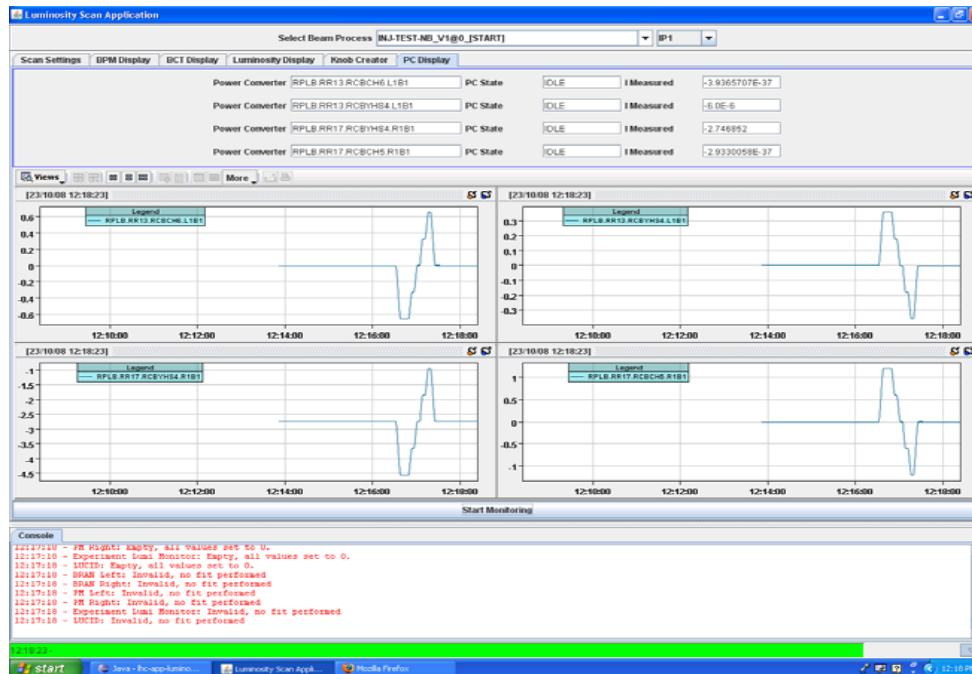
Screen shot of a dry run performed with the CCC application with nominal dI/dt.
