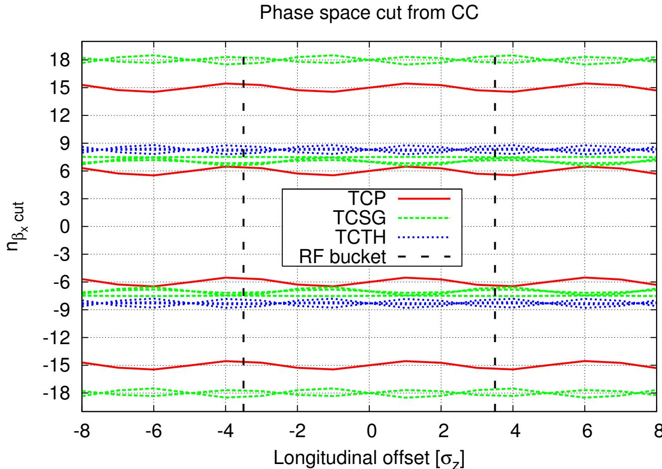
$D_{x,CC}$  and  $\beta_x$  being dependent of  $\delta_z$ , with primary, secondary and tertiary collimators
