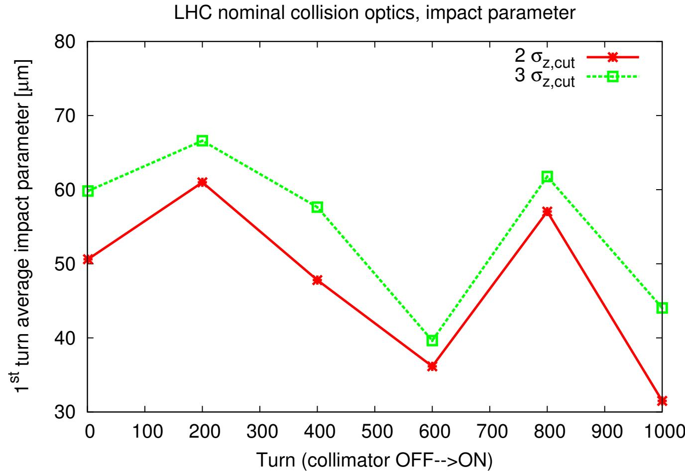
Collimators are turned **ON** at specified turn, then particles are tracked for another 200 turns, and get the '1st turn' impact parameter, **OFF-momentum + no CC**
