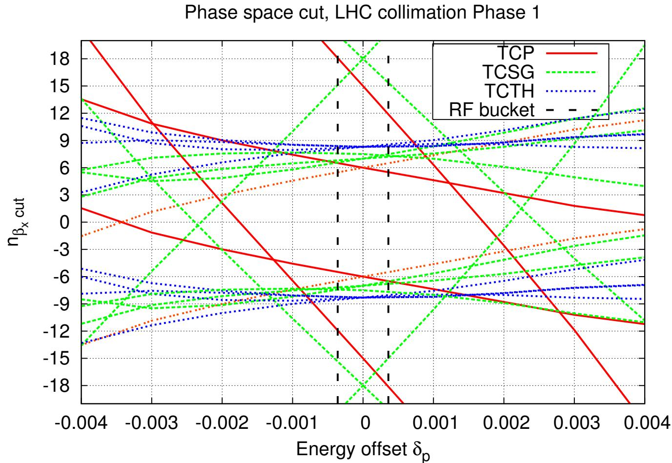
$D_x$  and  $\beta_x$  being dependent of  $\delta_p$ , with primary, secondary and tertiary collimators
