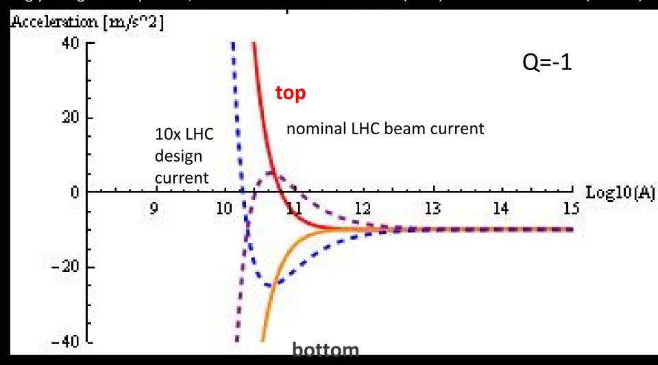
dust particles with masses larger than  $^{\sim}10^{11}$  proton masses can "fall" into the beam pipe, but the nominal beam cannot pick up any charged particles from bottom
