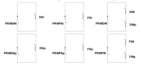
Narrow power converter circuit is separated for even and odd magnets: in total 7 power converters for 5 current mode (1 Figure of 8 loop + 6 PFW)
